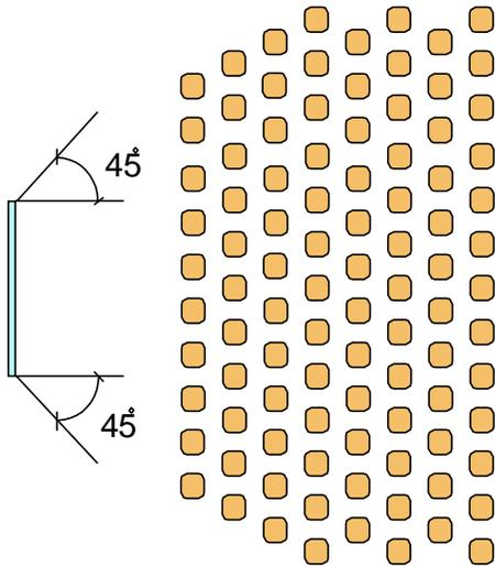
The **good** viewing area is within 45 degrees of the projection axis or within a 90 degree viewing cone.
