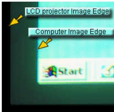
This is a photograph of an image that needs the horizontal and vertical position adjusted.
