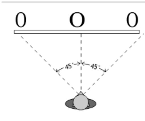
To determine viewing angles, it is a **best practice** to consider the least favoured viewer as being no further off-axis than 45 degrees from the farthest outside edges of the screen.
