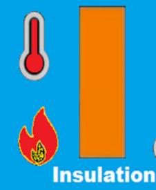
The ability of an element to resist heat transfer from the exposed face to the unexposed face
